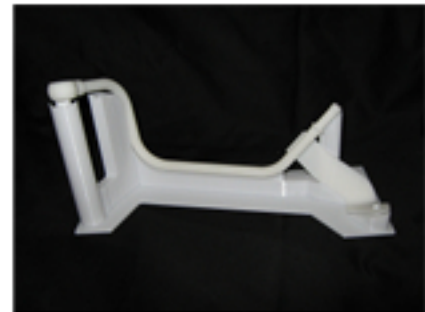
Figure 2: PC Test Fixture with ABS Trial Part
